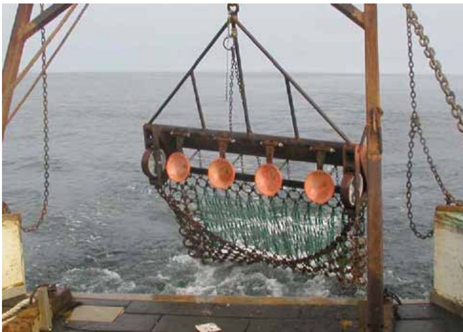
Figure 5. Prototype 8-foot hydrodynamic scallop dredge aboard the F/V Pretty Girl.
